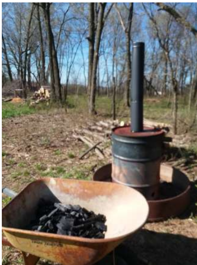
The Assembled Retort with the First Charcoal Produced.
